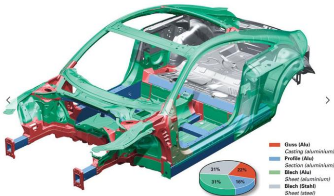
Fig. 4. Areas of application of aluminum in the construction of a car. Bodywork Audi TT made almost entirely of Al sheet (except the rear part of the body with reinforcements) [16]
