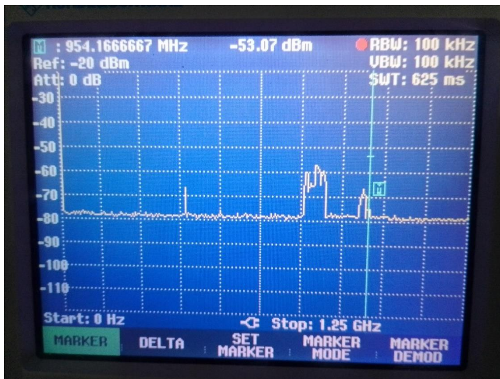
Fig. 2. The spectrum at frequency range between 100 kHz and 1.25 GHz. The level of the most powerful transmission is -53.1 dBm (at 954.17 MHz). The spectrum is measured when anechoic chamber's top cover is opened. Both resolution (RBW) and video (VBW) bandwidths are 100 kHz.
